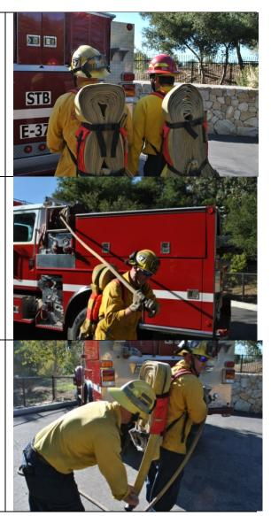
Engineer connects the 1½" trunk-line from the hose pack to the engine. This line becomes the trunk-line and will continue throughout the operation. Engineer prepares to charge the trunk-line. (Do not charge until they call for water.)
