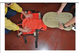
Tighten up the straps and put the bottom of the hose on the <u>stitching line</u> of the Modified Gasner Pack.
