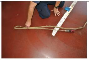
Continue to coil the hose in a circular motion. This is best done at the station (if possible) on the apparatus floor.
