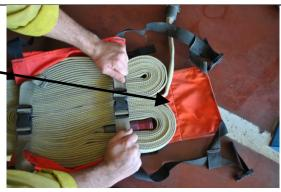
With the gated wye connected to the 1½" hose (as shown) leave a length of hose measured from your elbow to your finger tips, approximately 16-18". Start the hose load on the left side of the box (looking at the box from the open side).
