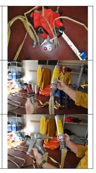
As an option in the station you can use the "SHOP VAC" to vacuum the air out of the hose. You will need tape, 1½" double male, and a reducer. This will create a vacuum much faster than the primer pump.
