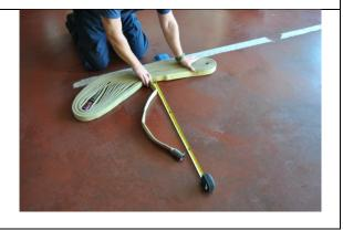
Lay the Modified Gasner Pack out flat on the surface with the clips fully extended. The 1" hose is always on the bottom of the pack. The tag end of the 1" hose will play out from the bottom of the pack.
